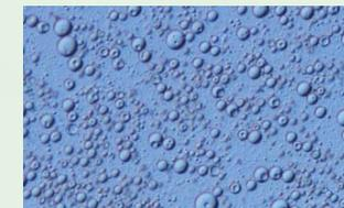
Particle size of cold/cold process with IMWITOR® 375.
